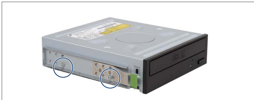
Figure 28: Attaching the EasyClick rails - example: DVD drive
